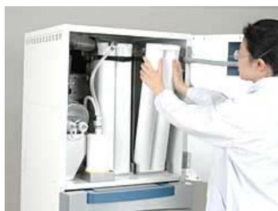
■ Most consumable parts, including the pretreatment cartridge and the ion-exchange resin cartridge, can be easily attached and detached, facilitating maintenance work.
